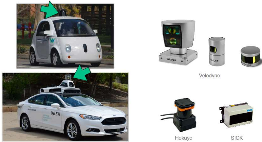
Figure 2.4 Typical LIDAR sensors and examples of mounting on various vehicles (Coursera (2019a))
