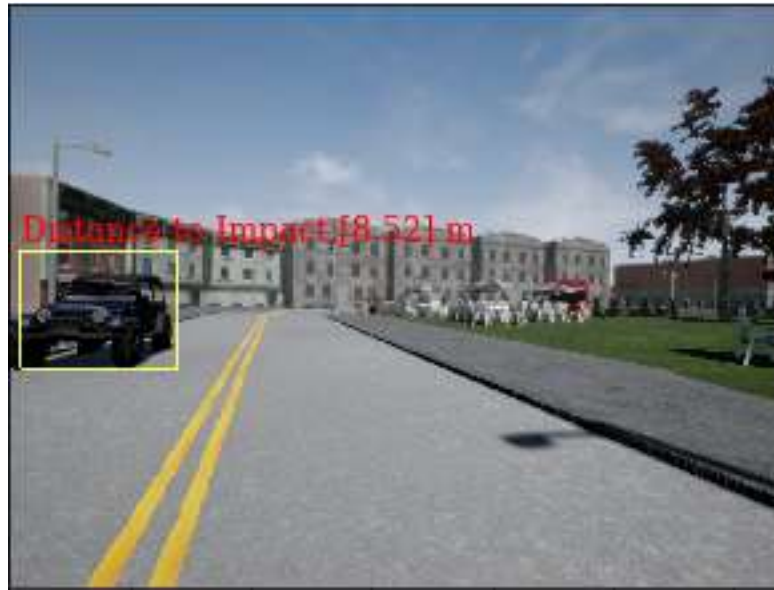
Figure 4.23 The distance between the center of the camera and the car (8.52m)
