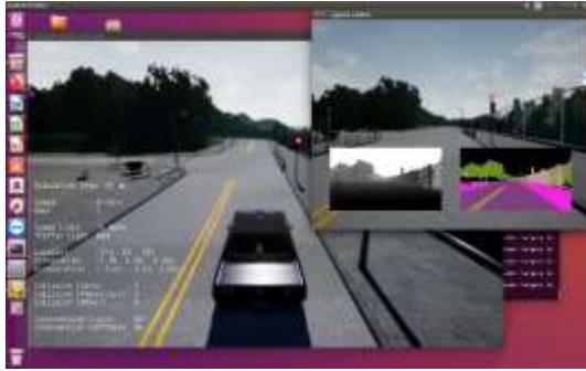
Figure 3.17 CARLA simulation environment with semantic segmentation and depth cameras (Screenshots from the DeOPSys Lab system)
