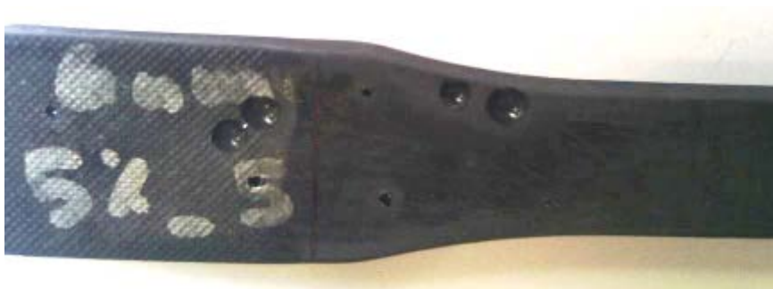
Figure 29: Epoxy nanocomposite with 5 wt% incorporation of GNPs showing bubbles in the surface.
