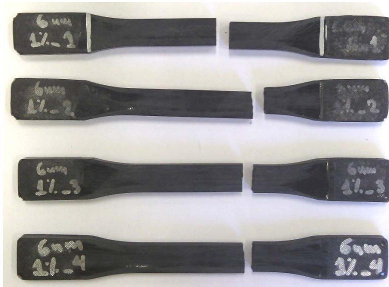
Figure 15: A tensile batch (four resin/GNPs specimens) after the conducted experimental procedure.
