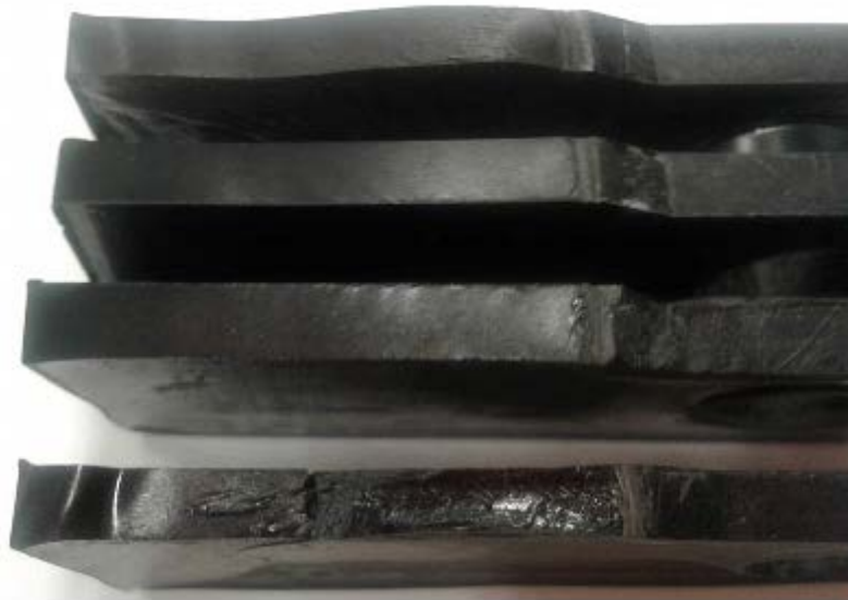
Figure 20: Fracture toughness specimens' surface areas after the experiment.
